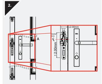
**a.** Insert the centre keep into the routed hole and ensure it sits flush to the face of the door frame.
