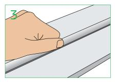
Fit inner sash, fit in parting bead (QW-CPB8) into clip profile (QW-SC1). Push and tap down until you hear the click
