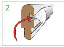
Cut parting bead to size. Slide seal (supplied separately) into finished parting bead (QW-CPB8).
