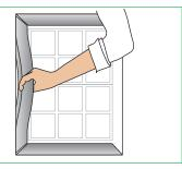
Bend centre of bead by hand and locate opposite end into clip profile at bottom corner mitre. Allow bead to snap back and tap down entire length until you hear the click. Repeat on other side.
