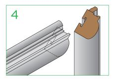
Measure sash frame and cut staff bead to size. Mitre cut top, bottom and side bead.
