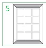
Fit outer sash, fit top and bottom staff bead (QW-CSB20) into clip profile (QW-SC1). Push and tap down until you hear the click.
