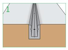
Machine grooves into sash frame to accept clip profile. Fit clip (QW-SC1) into groove, secure using pins or staples.
