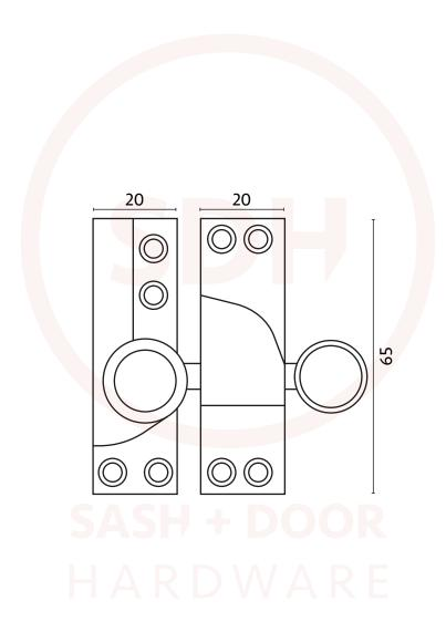
NOTE: This product is made from Cast Brass and manufactured using the Traditional Sand Cast method. The items requiring a Lacquer protection are protected using the Electrophoretically Lacquered process giving a very attractive long-lasting product.
